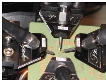
Figure 21. Step 2. Attach microprobes to the ends of the VNA cables Step 3. Perform all the measurements with microprobes
