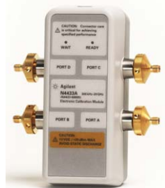
Figure 20. Step 1. Calibrate all ports at the end of the coax cable using the electronic calibration module
